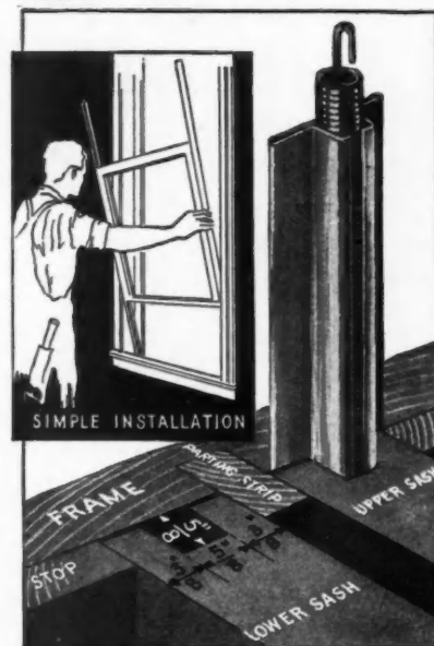
DETAIL SHOWING TYPICAL APPLICATION ON 1 1/8" SASH AND GROOVING DIMENSIONS
