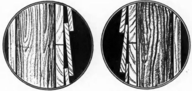
CLAPBOARDS, both square edge and bevel, came into use very early in our Colonial period. The original clapboards of this period still cover many old New England houses.
