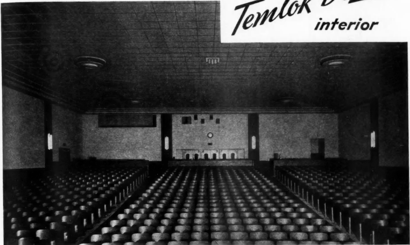
ATTRACTIVE PATTERN AND COLOR EFFECTS in the Foster Theater, Youngstown, Ohio, were obtained by using Coral Temlok De Luze Beveled Plank on upper walls and Ash Panels on ceiling. Pilasters and wainscot were finished in Armstrong's Temboard De Luze. Contractor: Heller-Murray Company, Youngstown. Scheibel and Shaffer, architects.
