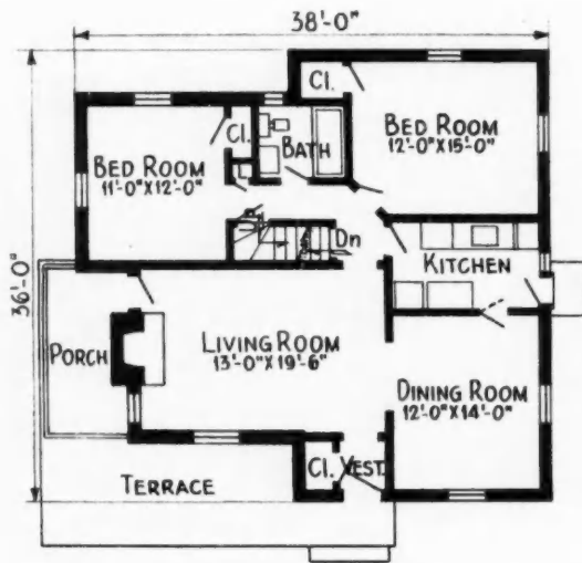
THE five-room bungalow above fulfills the continued demand for compact planning. It was designed by John D. Cobb, Washington, D.C., architect, and built in Northwood Park, Md., by Garden Homes, Inc. Maximum use of floor area, good circulation, terrace and living porch, and provision for extra bedrooms on the second floor are features.
