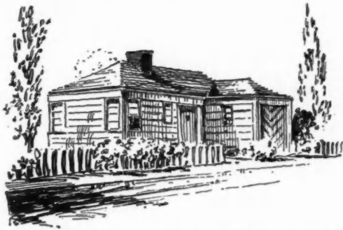
WIDE horizontal boards are also well suited to the modern home and particularly suit the long, low type of house. The pattern here illustrated was used on the Lumber Industries exhibit house at "A Century of Progress."
