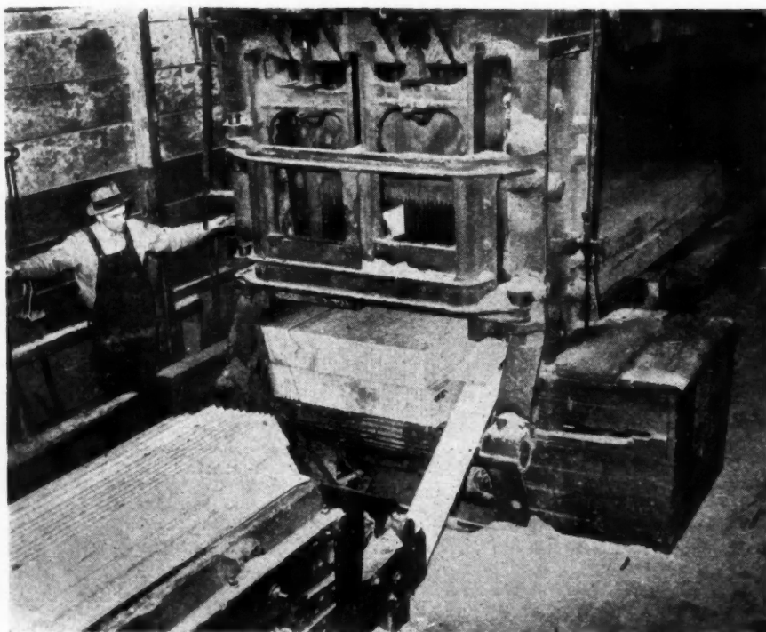
AN EXCEPTIONALLY fine picture of what is known as the gang saw. This machine is equipped with from 40 to 50 uniformly-spaced blades mounted on a reciprocating frame. These saws are run at 250 up-and-down strokes per minute so as to cut the cants into lumber which is the most uniform in size of all sawn wood.
