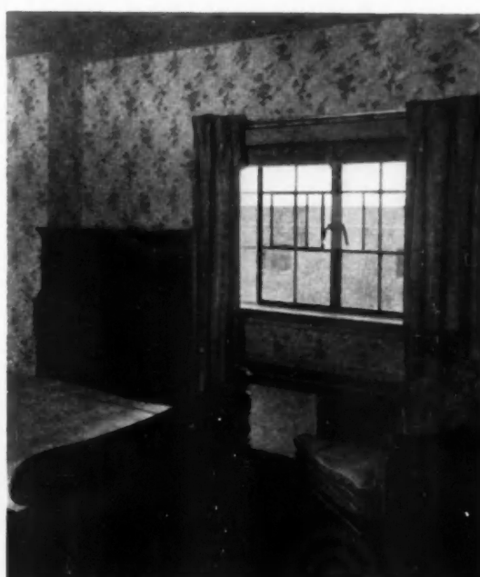
BEDROOM CORNER, showing space-saving convactor radiator, steel windows with screen, Venetian blinds.
