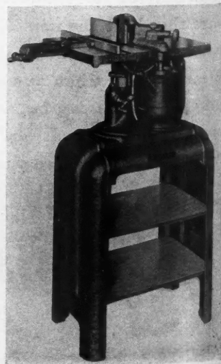
SHAPER has tilting table to allow added operations; extra heavy base makes it rigid.
