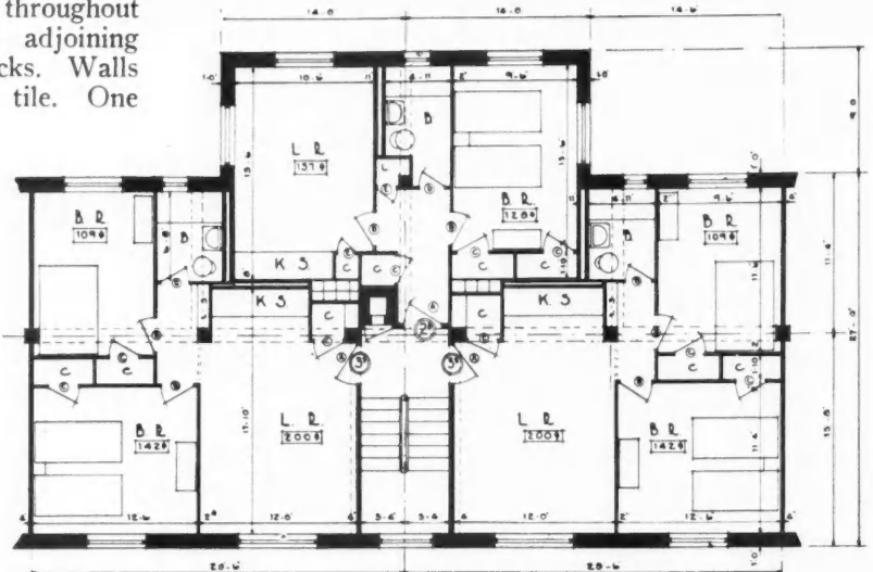
PLAN NUMBER HD-28; type of plan, T-unit; characteristics: plan with strip kitchens throughout, used as a ribbon, compulsory passing through living rooms in left and right apartments, no entry in left and right apartments, average room area increase due to the use of strip kitchens, 8 rooms in unit, total occupancy 13 persons, total gross area 1,791 sq. ft., average gross room area 224 sq. ft., total net area 1,187 sq. ft., average net room area 148 sq. ft., percent efficiency—gross vs. net area—66.3%, outside wall per room: 16 ft. 6 in. with no end wall, interior partitions per room 36 ft. 5 in.
