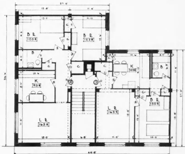
PLAN NUMBER HD-25; type of plan, corner unit; characteristics: bathrooms same throughout, used as a corner for joining of other plan types; not a very efficient unit because one stair and incinerator serves only two apartments per floor; 7 rooms in unit, total occupancy 8 persons, total gross area 1,462 sq. ft., average gross room area 209 sq. ft., total net area 899 sq. ft., average net room area 128 sq. ft., percent efficiency—gross vs. net area—61.5%, outside wall per room: 15 ft. 7 in. with no end wall, interior partitions per room 31 ft. 4 in.
