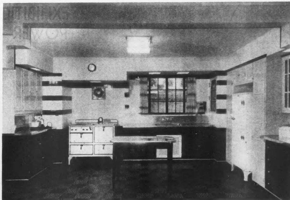
THE KITCHEN OF THE CENTURY —probably no section of the home reflects progress in layout, equipment and materials to a greater degree than does the kitchen. Above is illustrated a modern cook shop in Monel Metal, a modern industrial solid alloy of nickel and copper finding many household applications. This metal is used for the sink and for the cabinet, table and range tops. Color scheme is black, ivory, red—The International Nickel Co., Inc.
