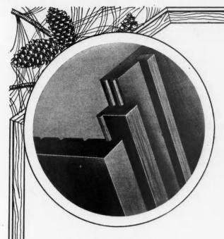
A double wedge-joint between pulley stile and blind stop, and a single wedge-joint between blind stop and casing, makes PINE CRAFT frames draft-proof, dustproof, weather-proof.
