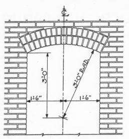
reinforced concrete lintels are called for. All such arches shall be rowlocked arches, segmental in form. Generally, one rowlock will be required for each twenty (20") inches in width of opening or fraction thereof. Radius of arches shall be equal to the width of the opening. The drawing shows a three (3) feet wide arch made to this specification. As the span is more than twenty (20") inches and less than forty (40") inches, two (2) rowlock lock arches are required.
