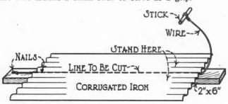
A Simple, and Accurate Method of Cutting Corrugated Iron with a Wire.
