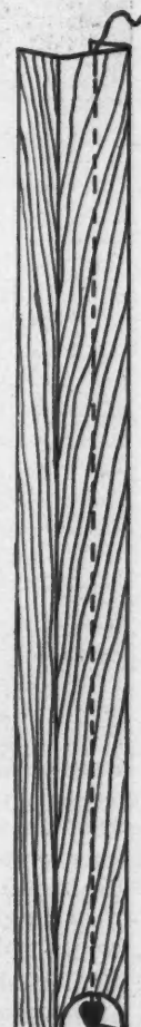
With the Plumb Bob Hung in a Box Like This the Wind Does Not Affect It.
