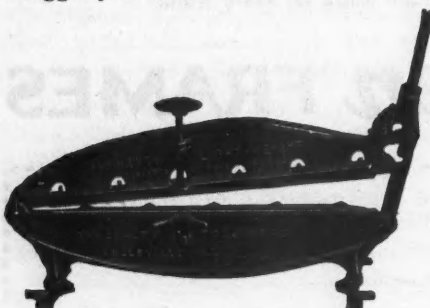
This Light Shingle Cutter Is Easily Handled on the Roof, But Is Very Effective.
