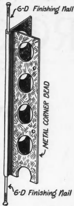
If This Method Is Used Short Pieces of Corner Bead Need Not Be Wasted.
