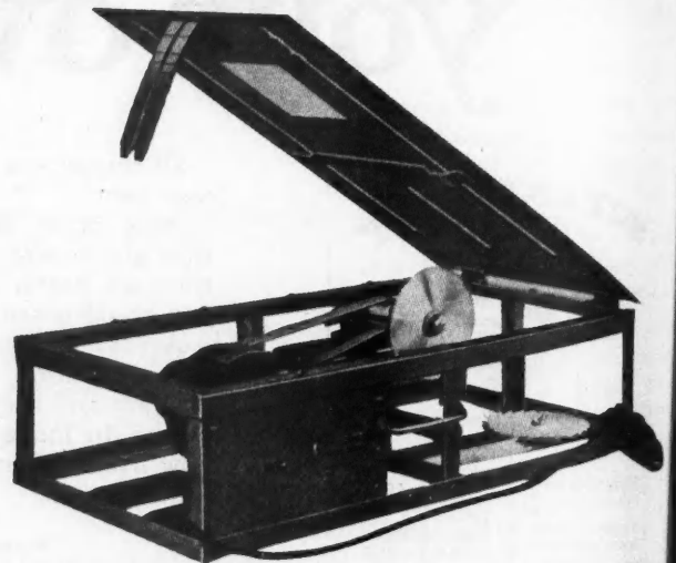
A Thoroughly Efficient Saw Which Is Self-Contained and Can Be Carried Like a Piece of Baggage Where Desired.
