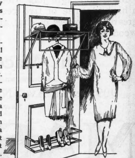
Two Simple Fixtures May Be Attached to the Door of the Closet to Greatly Increase Its Capacity and Neatness.
