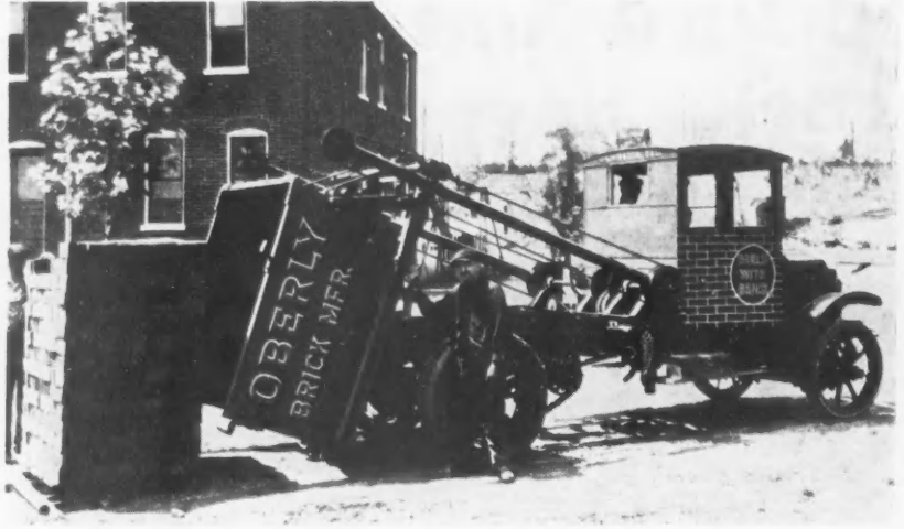
The Body Is Lowered Over an Arc, Depositing the Brick in a Neat Hack on a Wooden Pallet, the Whole Operation Requiring Only Three to Five Minutes.
