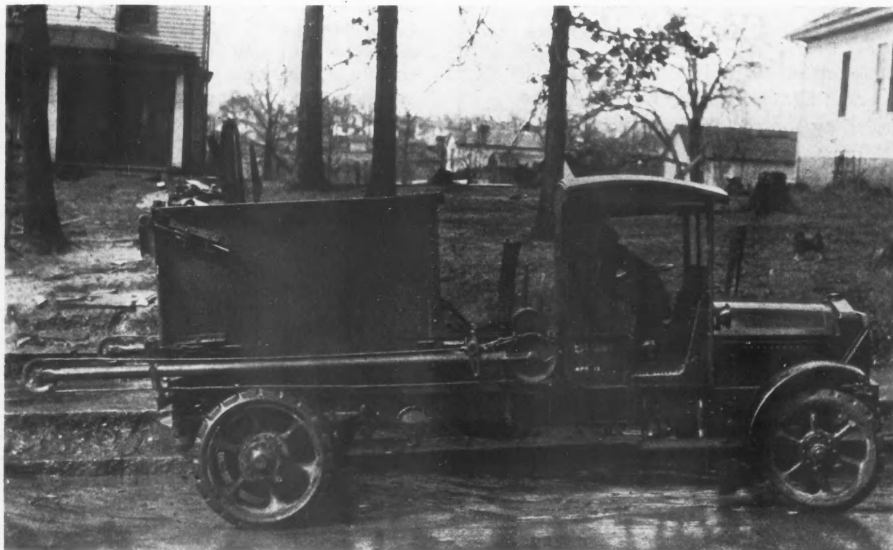
This Special Body for Handling Brick and Similar Building Materials Can Be Mounted on a Short Wheel Base Chassis Which Is Easily Handled Under Difficult Conditions and Permits the Depositing of the Material at Any Desired Point Without Breakage.
