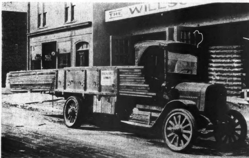
Special Bodies and Quick Unloading Devices Are Used by Lumber Dealers and Contractors.
