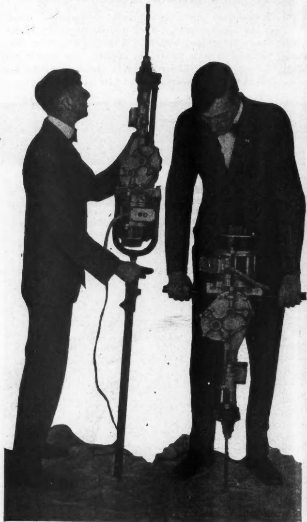
This Portable Concrete Drill Makes the Drilling of Floors, Walls and Ceilings a Quick, Simple Matter. Weighs 56 lbs. Driven by electricity and compressed air.
