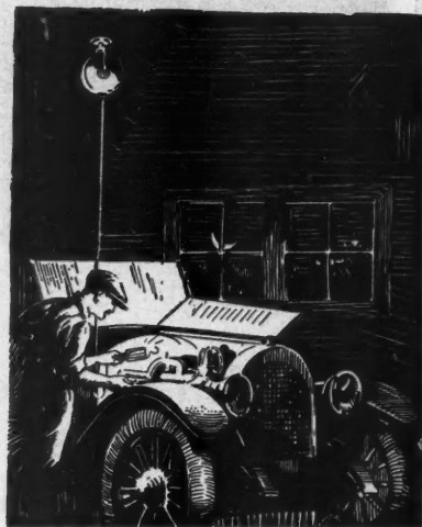
This Man Lights His Work with a Lamp Reeled Down from Overhead; It Is on a Spring Roller.
