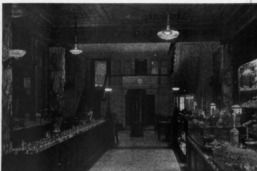
Fig. 4. Semi-Indirect Lighting. This is an excellent example of the artistically illuminated shop, the tinted shades softening the light in a way that avoids all bare, glittering and garish effects. A cool light for cool shop, for this is Schraft's Candy Shop, 38 Fifth Avenue, New York City.
