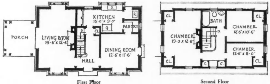
First and Second Floor Plans of Brick Colonial House in which Steel Lumber Joists Were Used.
