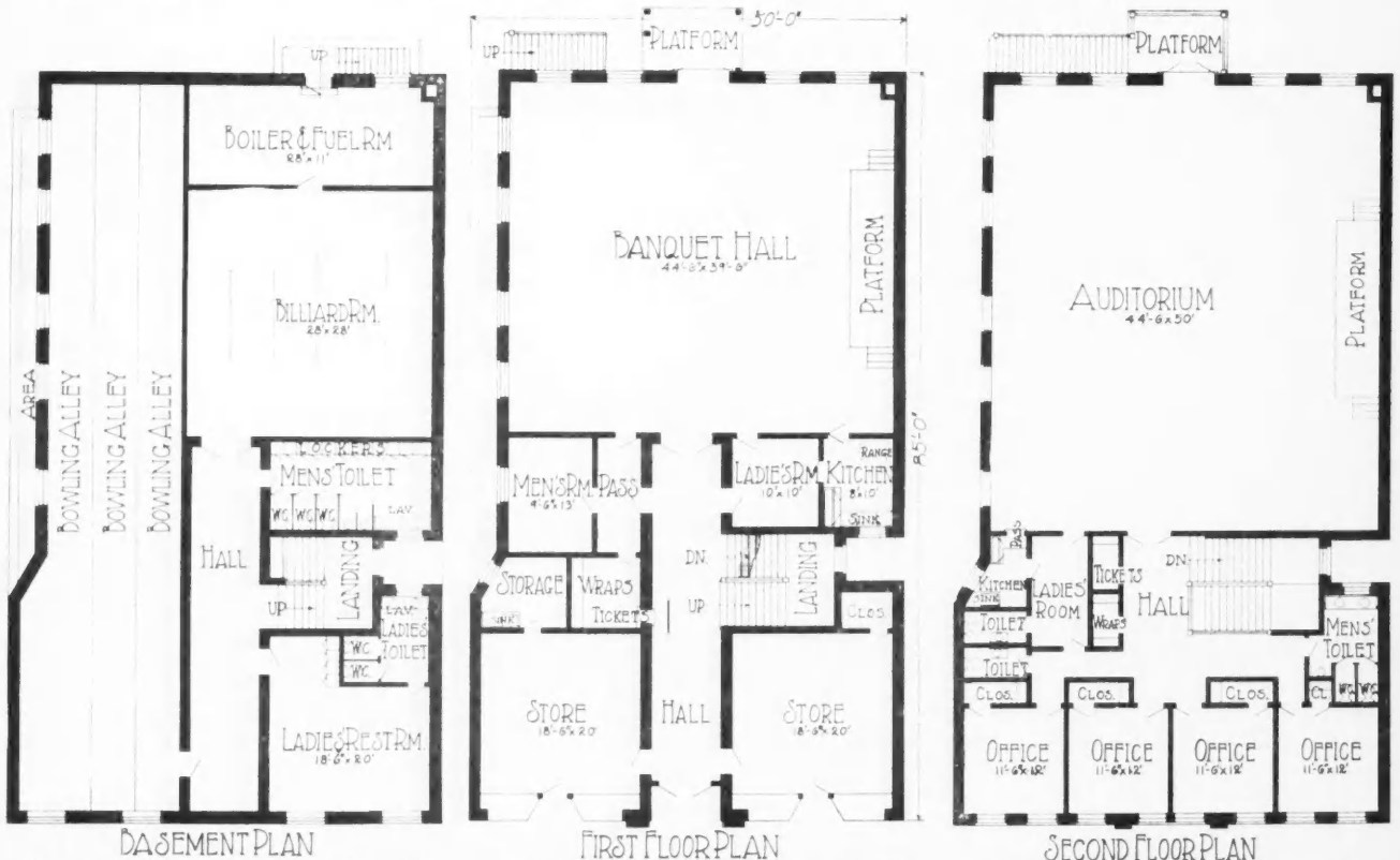
Basement Plan of Proposed Community Hall, Showing Recreation Rooms, Bowling Alleys and Maintenance Section.
