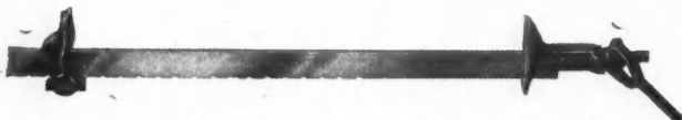
Utility Clamp for Cabinetmakers and Joiners with Special Handle. It Is Tightened by Pulling the Screw and Bar Thru the Front Casting.
