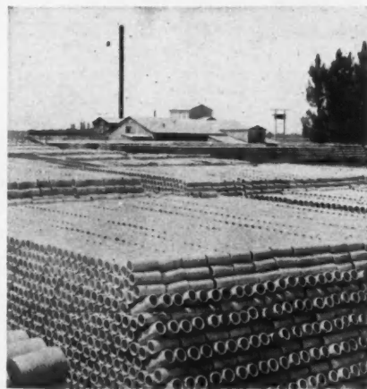
Two Hundred Fifty Thousand Lengths of Concrete Drain Tile Ready in the Spring for a Busy Season. Concrete Tile May Be Made All Winter Under Conditions Similar to Those Described in the Accompanying Article for the Year 'Round Manufacture of Blocks.
