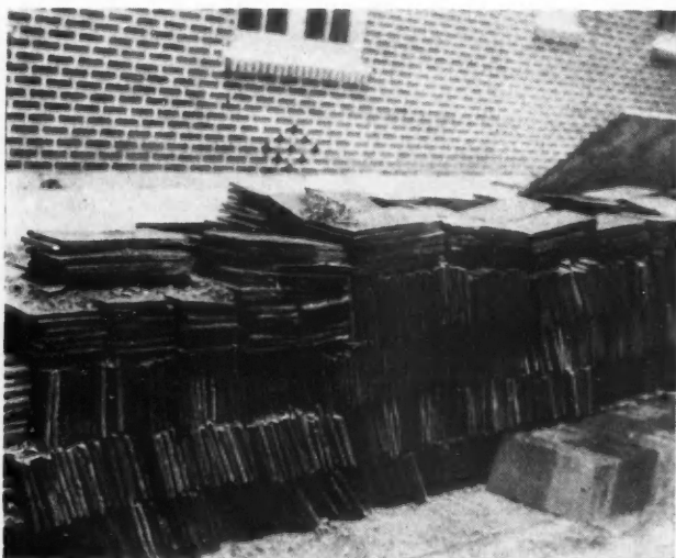
Close-Up View of Pile of Brick Shingles Which Were Used in Simon Home. They Are Made of Clay Like Ordinary Brick But Moulded Thinner.
