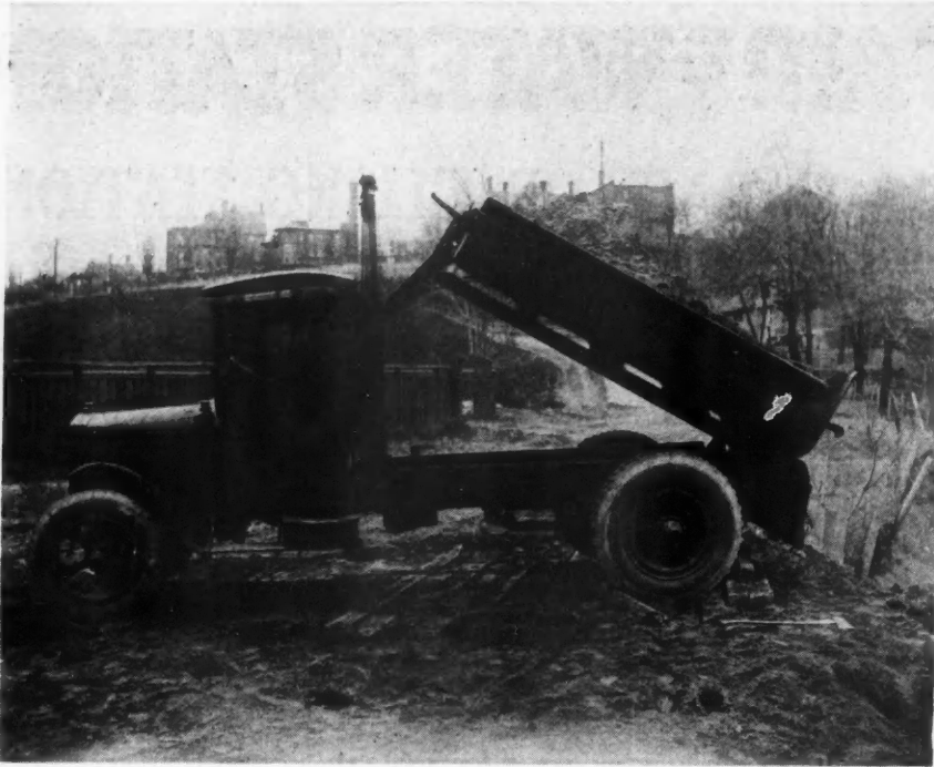
Mr. Plummer, Excavation Contractor, Minneapolis, Minn., Says This 3 1/2-Ton "Acme" Does the Work of Seven Teams. Here It Is Shown Dumping One of the Many Loads of Dirt It Carries Every Working Day. It Averages About 90 Miles Per Day Over a Loose, Sandy Road.
