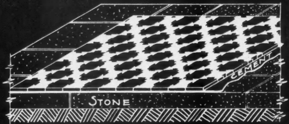
LAID OVER STONE FLOOR
