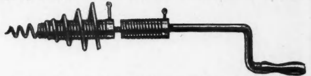
Corkscrew Arrangement at End of Flexible Wire Closet Cleaner. This Catches Any Obstruction Which May Be Lodged in Drain or Trap.
