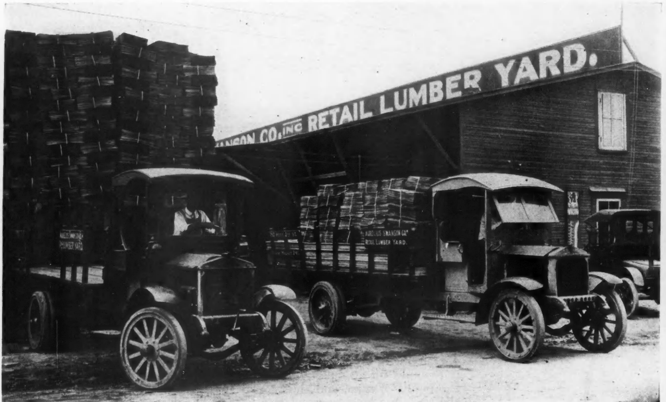
The Retail Lumber Yard and the Two 2-Ton "Federal" Trucks Operated by the Aurelius-Swanson Lumber Co., Oklahoma City, Okla. The Two "Federals" and the Light Delivery Car Handled $250,000 Worth of Lumber in 1918, Replacing 15 Teams and Wagons and Cutting the Delivery Costs of the Company 40 Per Cent.
