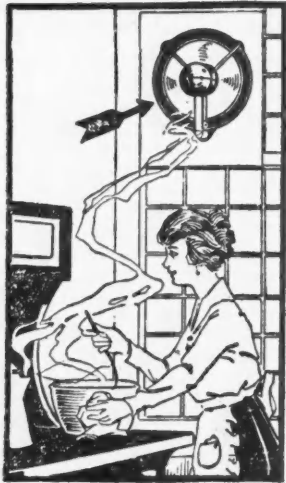
An Electrically Operated Ventilator Set in the Glass of the Kitchen Window Sucks Out the Cooking Odors and Keeps the Air in the Room Fresh.
