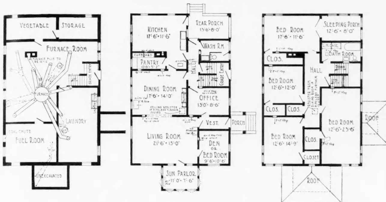
Basement Plan. First Floor Plan. Second Floor Plan. Arrangement of Farm House, Design No. 6887, Illustrated on Opposite Page. Size on the Ground, 32 by 48 Feet.
