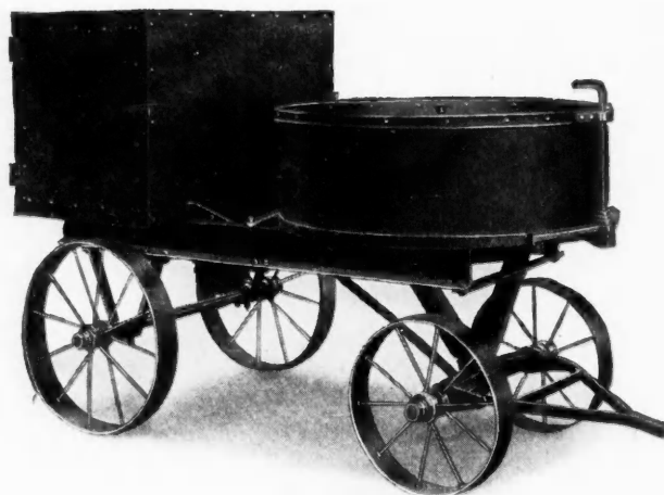
Showing the "Frank" Concrete Mixer and Housed Gasoline Engine Mounted on Truck.
