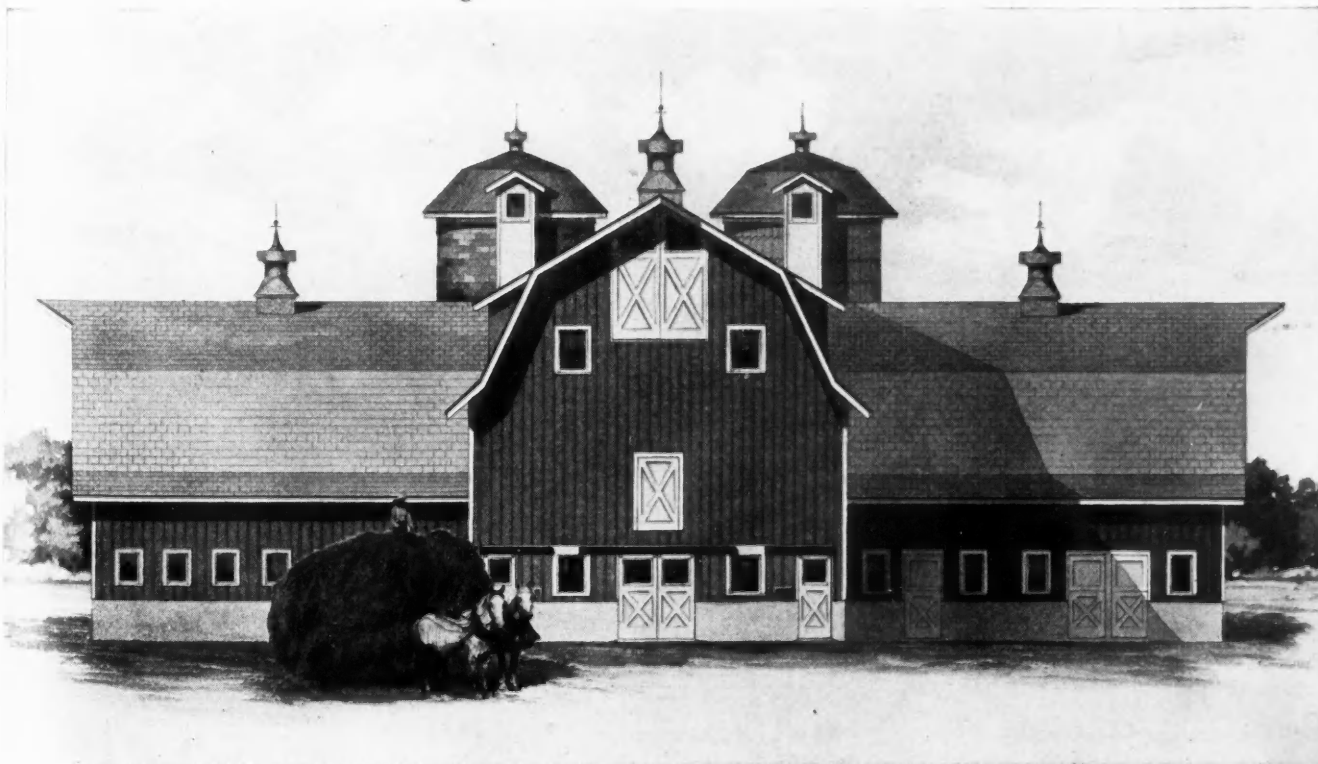
Front View of Large General Barn. The form in which this Barn is planned, gives it an impressive, distinctive appearance from every point of view. The dairy stable is in the main section; the horse barn the left wing, and the stock or calf barn the right wing. For floor plans and details of construction, see Pages 57 to 61.
