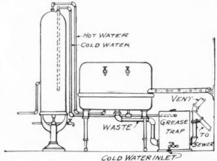
Fig. 2. Grease Trap for Kitchen Sink. The Cold Water Pipe Cools the Grease so It Can be Removed.
