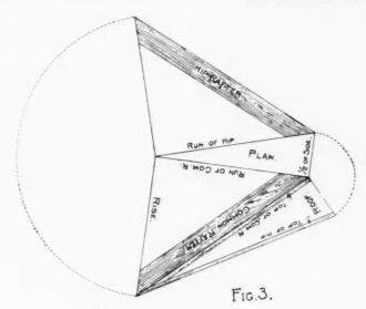
Fig. 3. Diagram Showing How to Lay Out Model for the Framing of the Roof.
