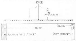
Fig. 2B. Freely Supported Beam with a Concentrated Load at Center of Beam.
