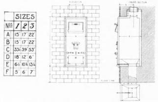
The Built in the Wall Type of "Incinerite."
