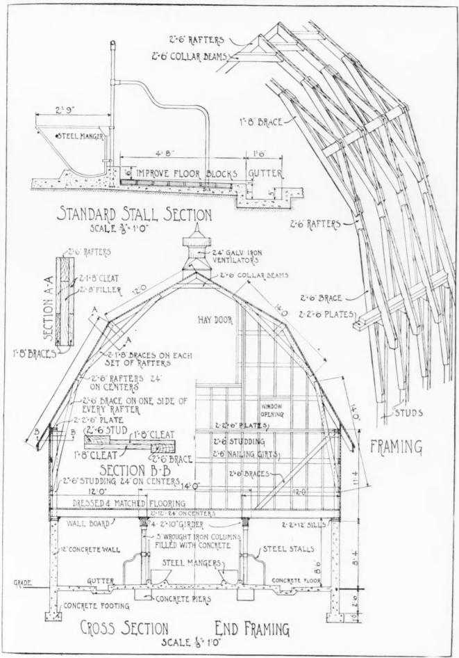
Details of Plank Frame Gambrel Construction in which Every Rafter is a Truss, Leaving Hay Mow Entirely Clear. Half of Cross Section View Shows End Framing. Design No. A299 Illustrated on Opposite Page.
