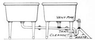
Fig. 1. Laundry Tubs, Showing Ordinary Trap. The Vent Pipe Prevents Gases from Escaping Into the House.
