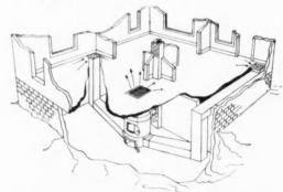
Cn(-Away Section of House Showing Operation of Kalamazoo Pipeless Furnace.
