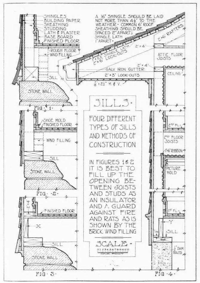
Scale Details by E. T. Huddleston, Architect, Showing Four Typet of Sill Construction. For Description See Opposite Page.
