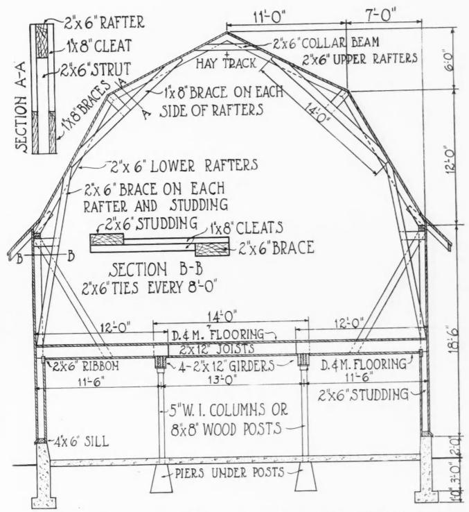
Detail Showing Recommended Sizes for Various Members in Plank Frame Barn That Is 36 Feet Wide.
