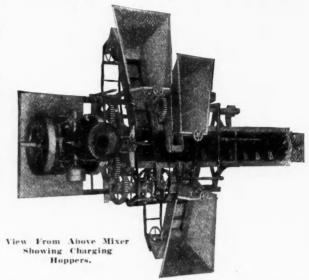
on these mixers. The grates can be raised or lowered to give the proper proportions for either the sand or stone with regard to the amount of cement used. The gates are hinged so that large stones can pass thru without breakage and the springs hold it in place.
