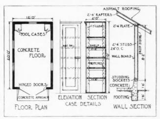
Details of Garage G160. Showing Floor Plan and Method of Constructing Walls and Tool Cases.
