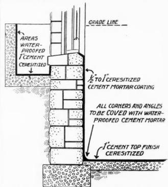
Waterproofing Basement and Area Walls with a Ceresitized Cement Mortar Coat.
