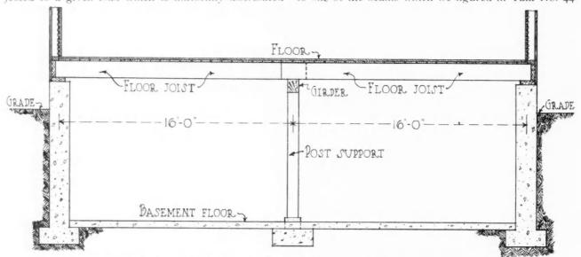
Fig. 2A. Beam with Uniformly Distributed Load, Ends of Beam Freely Supported.
