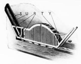
Substantially Built Safety Guard for Saw Table.
