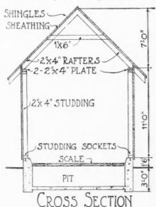
Dimensioned construction view of scale house.
