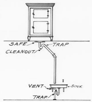
Fig. 3. Method of Constructing Waste Pipe for Refrigerator. The Pipe Should be Cleaned Regularly with Boiling Water.
