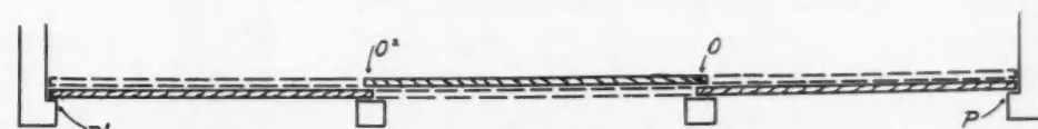
Fig. 8. Group of Three Parallel Doors which Require Bolt at "O" and Locks at "P" and "P"
