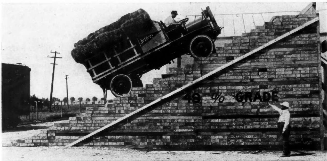
Scarcely an Ideal Road for Heavy Hauling; But This New Style Truck, Having Power Drive on All Four Wheels, Handles it Successfully.
