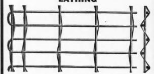
ELIMINATES ONE-HALF OF INSTALLATION COST, owing to its Truss formation, which makes it possible to staple or nail it directly to studs or joists without furring.
