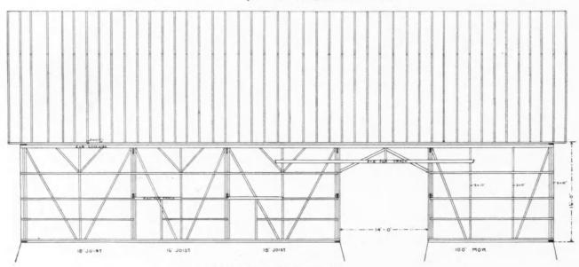
SIDE ELEVATION SHOWING FRAMING
