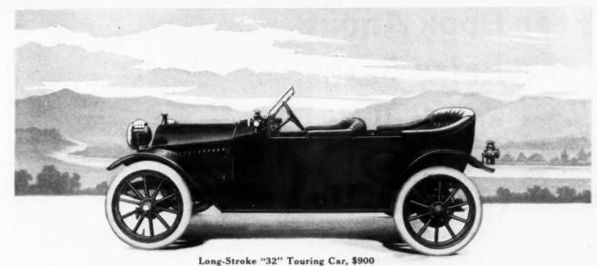
F. O. B. Detroit, including equipment of windshield, gas lamps, and generator, oil lamps, tools and horn. Three speeds forward and reverse; sliding gears. Four cylinder motor, 3½-inch bore and 5½-inch stroke. Bosch magneto. 106-inch wheelbase; 32x3½-inch tires. Color, Standard Hupmobile Blue. Roadster, \$900.
