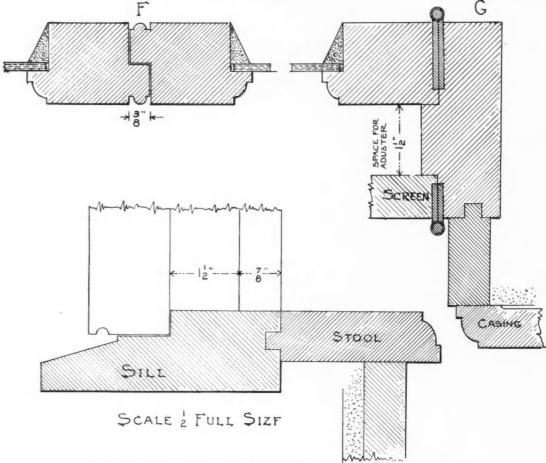
DETAIL NO. 12—STANDARD DETAIL FOR OPEN OUT CASEMENT WINDOWS
