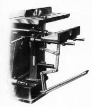
This attachment converts the borer into a hollow chisel mortiser, suitable for cutting mortises up to % inch
