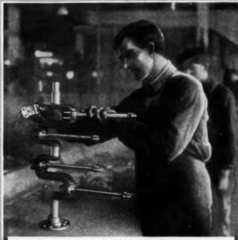
Here is shown the assembly of crankshaft and connecting rods; and the careful adjustment of the connecting rod bearings. Please note the center main bearing and the extra-generous length of the two end bearings. A third crankshaft bearing is unusual in a motor cast en bloc, except in cars of \$2500 or higher. So, in the \$900 Hupmobile, the crankshaft has three instead of two supports to help it withstand the strains to which this part necessarily is subjected.
