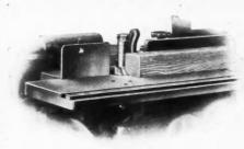
Poles and shafts can easily be rounded on the shaper spindle. This feature will appeal to the wagon and carriage builder. All you need to do this work is the special knives.
