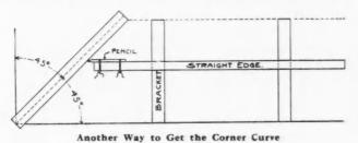
angle of 45 degrees. Then I took a straight edge and fastened a pencil on the end of it and by passing the straight edge over the face of the common brackets and with the pencil end against the angle piece, in that way described the required curve for the angle bracket. Get 'em?
