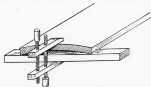
Hand Screw to Straighten Warped Boards
