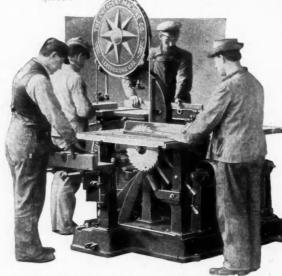
Four men can work on the No. 51 CRESCENT Universal wood worker without interfering with each other. Each machine may be started and stopped independent of any other and each workman controls his own work.
