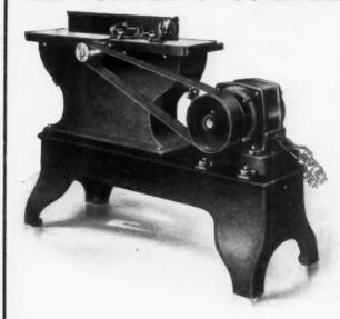
Is used for Jointing, Planing, Moulding, Beveling, Rabbeting, Grooving, and any other work that any Jointer can be used for. We furnish it with or without countershaft, bench or motor. Just as you desire. The **Best** machine for the money on the market. We make 6 larger sizes, and Wood Lathes, Shapers, Planers, Cut-off Saws, Band Saws and Saw Tables.
