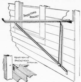
Sheathing Bracket, Designed to Pull Down, not Out
