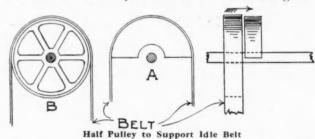
off onto the false or dead half pulley, the belt being shoved off the pulley on to the crib or false pulley in the direction of the arrow.
