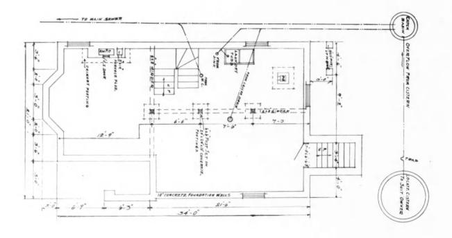
BASEMENT AND FOUNDATION PLAN AND REAR ELEVATION (House, Page 59)
