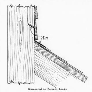
bottom where it begins. Where there is only lap siding, I cut a short slanting kerf in the studs to catch the water, running down same and insert the upper edge of the tin in same as shown.
