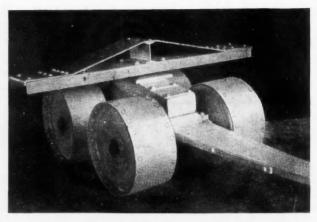
Fig. 4 Showing Steel Bolster on La Plant 4-Wheel Truck
