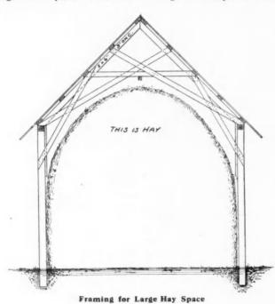
storms, and more so when it is empty; even at best only the ordinary windstorms that prevail every season can be taken into consideration. How best to place the bracing is the question, so as to give the least interference with the stacking of the hay.
