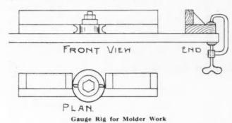
a tread; if there was no gauge, the tread would run in too far and spoil it. Here is an illustration for the gauge for treads and such like.
