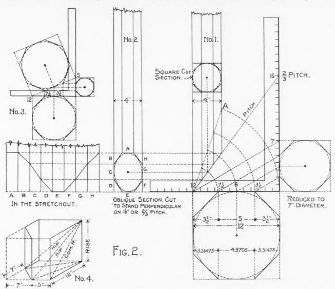
draw other lines from  $7\frac{1}{2}$  and  $3\frac{1}{2}$  and where these lines intersect the blade will be the points from which to develope the octagon, as shown. By the mental system it is 5 by 7 equals 35, which in this case is equal to thirty-five twelfths inches or 2 II/I2 inches to the side.
