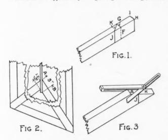
rafters are 45 degrees and equal pitches. Now, I claim that it applies to any angled building with unequal pitches, as shown at Fig. 2. Measure the distance on the plan from A to B and apply as shown by Ashley in Fig. 1. Suppose 2 or 3 inches is wanted on a level, then cut at top of rafters as shown at A, Fig. 3, which is the same as the foot cut, then set bevel to the angle on plan and apply as shown. It is a good thing to understand these points because it means a more efficient workman,
