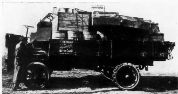
Speedwell with Seat Raised, Showing Accessibility of Motor
