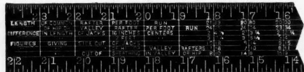
The Nicholls Rafter Framing Scale
