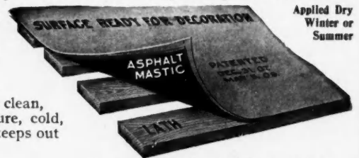
Shows Construction of Bishopric Wall Board
