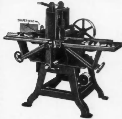
Universal Wood Worker, equipped with our Planing Attachment, will plane up to 4 in. thick and 10 in. wide; also arranged for doing two side molding, matching and sticking.
