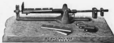
No. 1 Knife Balancing Machine
