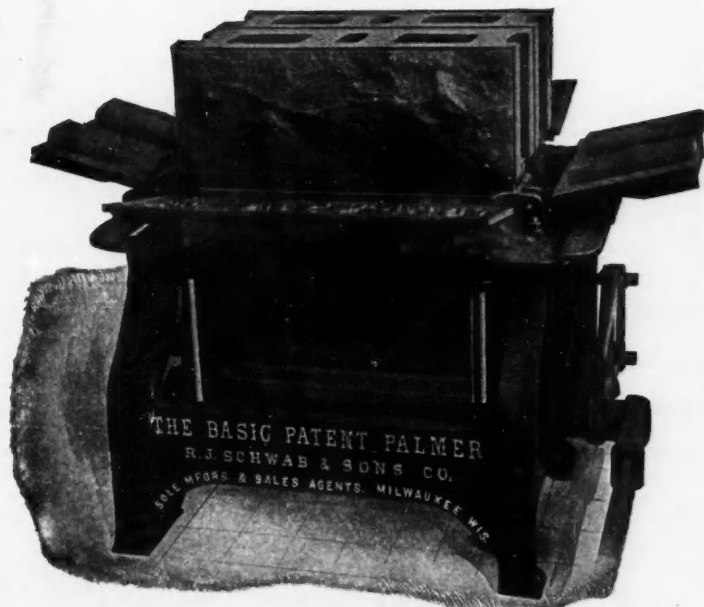
Showing Machine Open With Two Blocks Made at Once Ready for Removal
