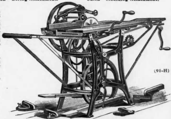
No. 5 "Union" Combination Self-Feed Rip and Cross-Cut Saw.
